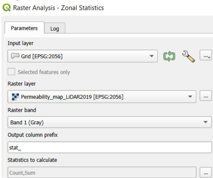
After execution, a new layer will be created, identical to the starting grid and containing new columns with the calculated statistics:
