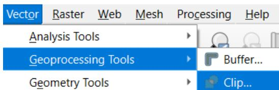
This will open the algorithm window in which you need to enter the grid as input, the municipalities layer as overlay and (optionally) choose a location for the output file:
