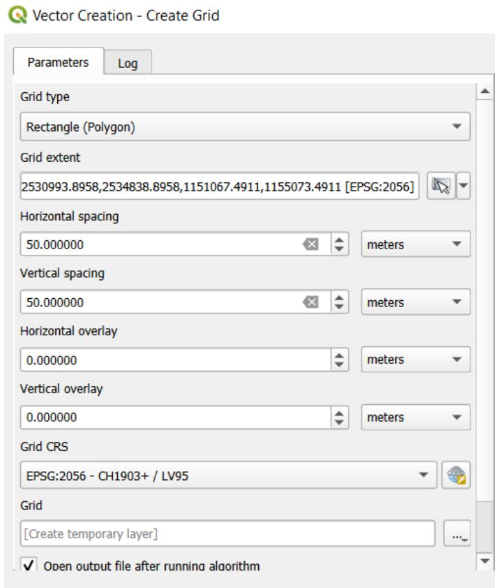
Make sure you select the `communes_ex2` layer for the Grid extent parameter and the correct coordinate system for the Grid CRS.
